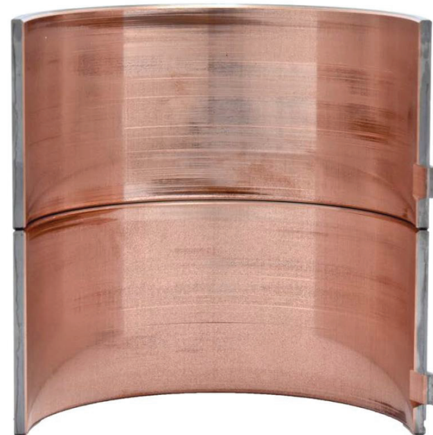
Rod Bearing, Fail
