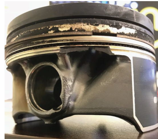
Piston damage due to preignition events
