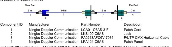
Standard(s)/Specification: ANSI/TIA-568.2-D Category 6A and ISO/IEC 11801-1 Class E<sub>A</sub> with the applicable electrical transmission characteristics
